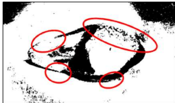
Figure 15: Distribution of Disconnected Pixels along the Boundary of an Impact Mark
