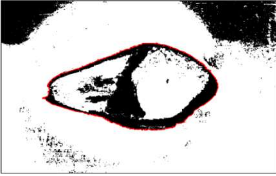
Figure 19: Identified Largest Contour (Highlighted in Red) Enclosing the Bullet Impact Mark
