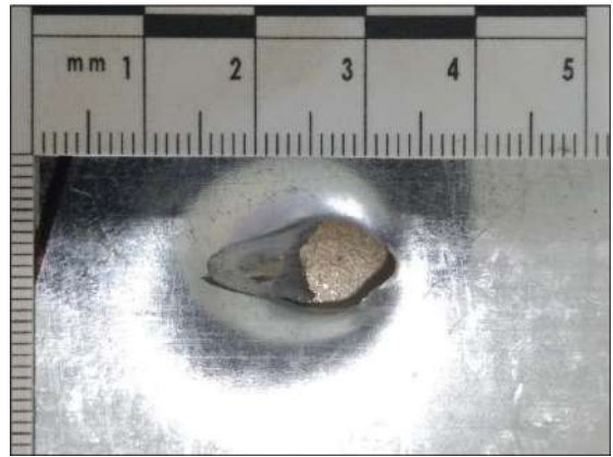
Figure 7: A Digitised Firing Data at a 30^\circ Incident Angle, with a Forensic Ruler Positioned Adjacent to the Bullet Impact Mark
