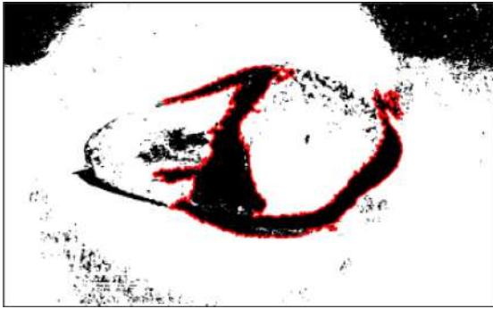
Figure 16: Erroneously Marked Outline (Highlighted in Red) Caused by Disconnected Pixels Along the Impact Mark's Boundary
