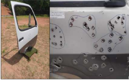
Figure 21: Firing Data Samples on a Van Door Manufactured from 1 mm Zinc-Coated Sheet Metal
