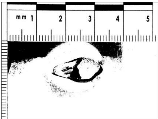
Figure 11: Noise Filtered Binary Representation of a Bullet Impact Mark at a 30° Incident Angle
