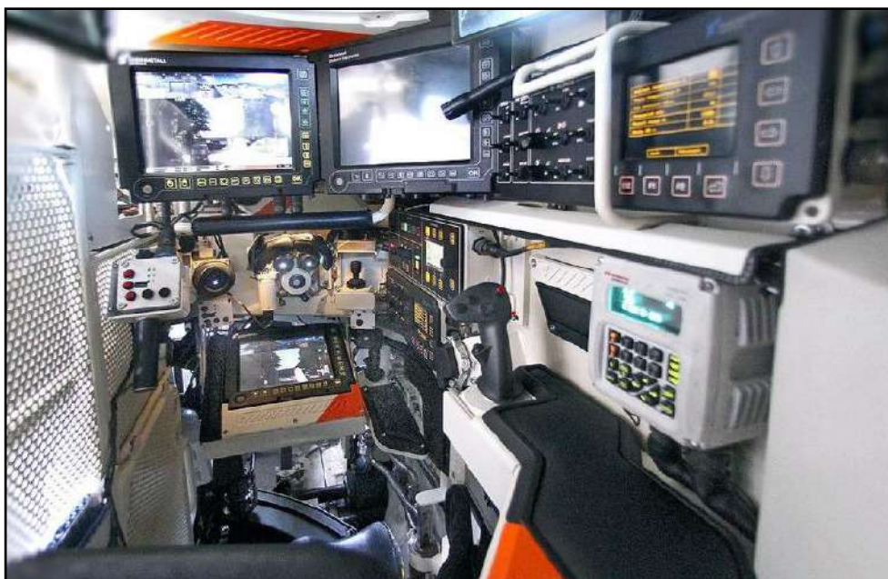
Figure 1.13: Leopard 2A7 tank inside with BMS
