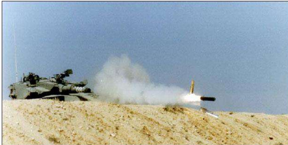
Figure 1.4: Merkava 4 launching LAHAT ATGM from smoothbore gun
