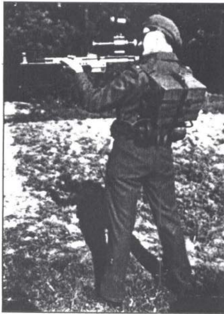
The German 'Vampir' infra-red night sight being tested by a British soldier in 1945. Note the size of the back-pack which contained batteries for the IR searchlight and compressed gas for cooling the IR detector in the sight unit.
